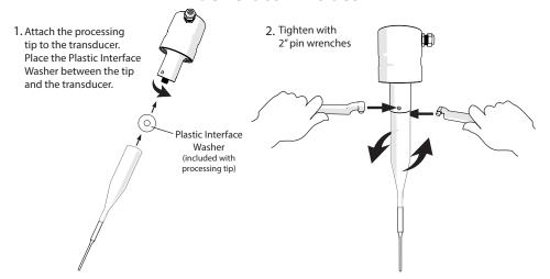
**CAUTION:** Use wrenches to twist the processing tip. Do not twist the Transducer.
