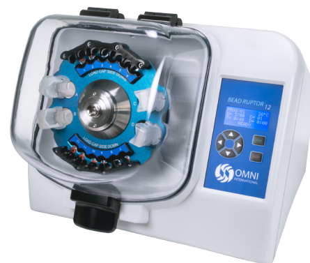
Figure 2. Omni Bead Ruptor 12 delivers reproducible results for high throughput sample homogenization of heart tissue.
