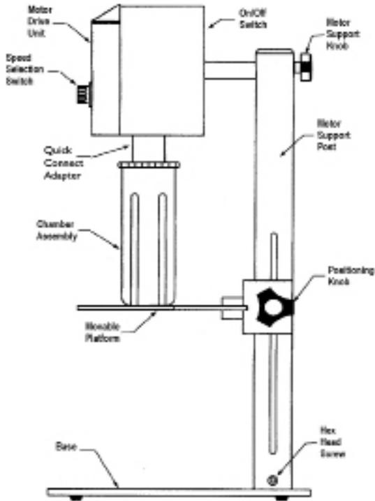
**WARNING:** When using sealed chamber assemblies, the bottom of the chamber assembly must rest on the movable platform. This prevents the chamber assembly from disengaging from the motor, which could expose rotating blades, and could lead to a broken seal.
