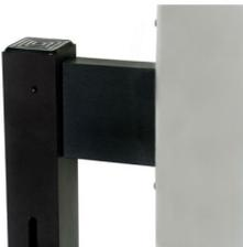
4. Seat the MES motor unit fully against the post before adding the Threaded Knob.
