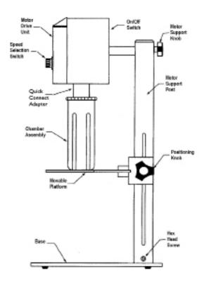
**WARNING:** When using sealed chamber assemblies, the bottom of the chamber assembly must rest on the movable platform. This prevents the chamber assembly from disengaging from the motor, which could expose rotating blades, and could lead to a broken seal.
