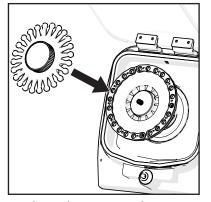
**3.** Place the Finger Plate on the Bead Ruptor Elite™ Hub.
