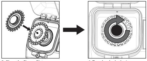
**3.** Place the Finger Plate on the Bead Ruptor Elite™ Hub.
