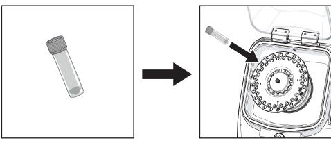
**1.** Fill tube with sample for processing.
