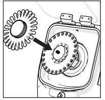
**3.** Place the Finger Plate on the Bead Ruptor Elite<sup>™</sup> Hub.
