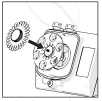
**3.** Place the Finger Plate on the Bead Ruptor Elite<sup>TM</sup> Hub.
