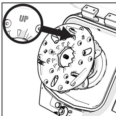
**2.** Place the 50 mL tube carriage on the Bead Ruptor Elite™ Hub as shown.
