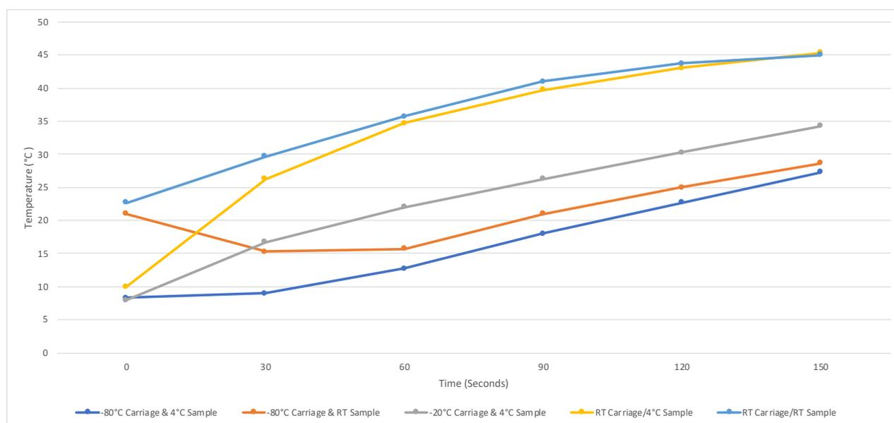
Samples remained the coldest when processing in the carriage equilibrated at  $-80^{\circ}\text{C}$  compared to carriages equilibrated at  $-20^{\circ}\text{C}$  or room temperature. Using chilled buffers alone did not keep samples below  $15^{\circ}\text{C}$  during the first 30 seconds of processing. Using cooled buffers in combination with a carriage equilibrated at  $-80^{\circ}\text{C}$  provided the coldest recorded samples at all tested time points.
