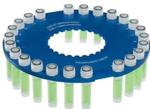
**Bead Ruptor Elite™ Bead Mill
